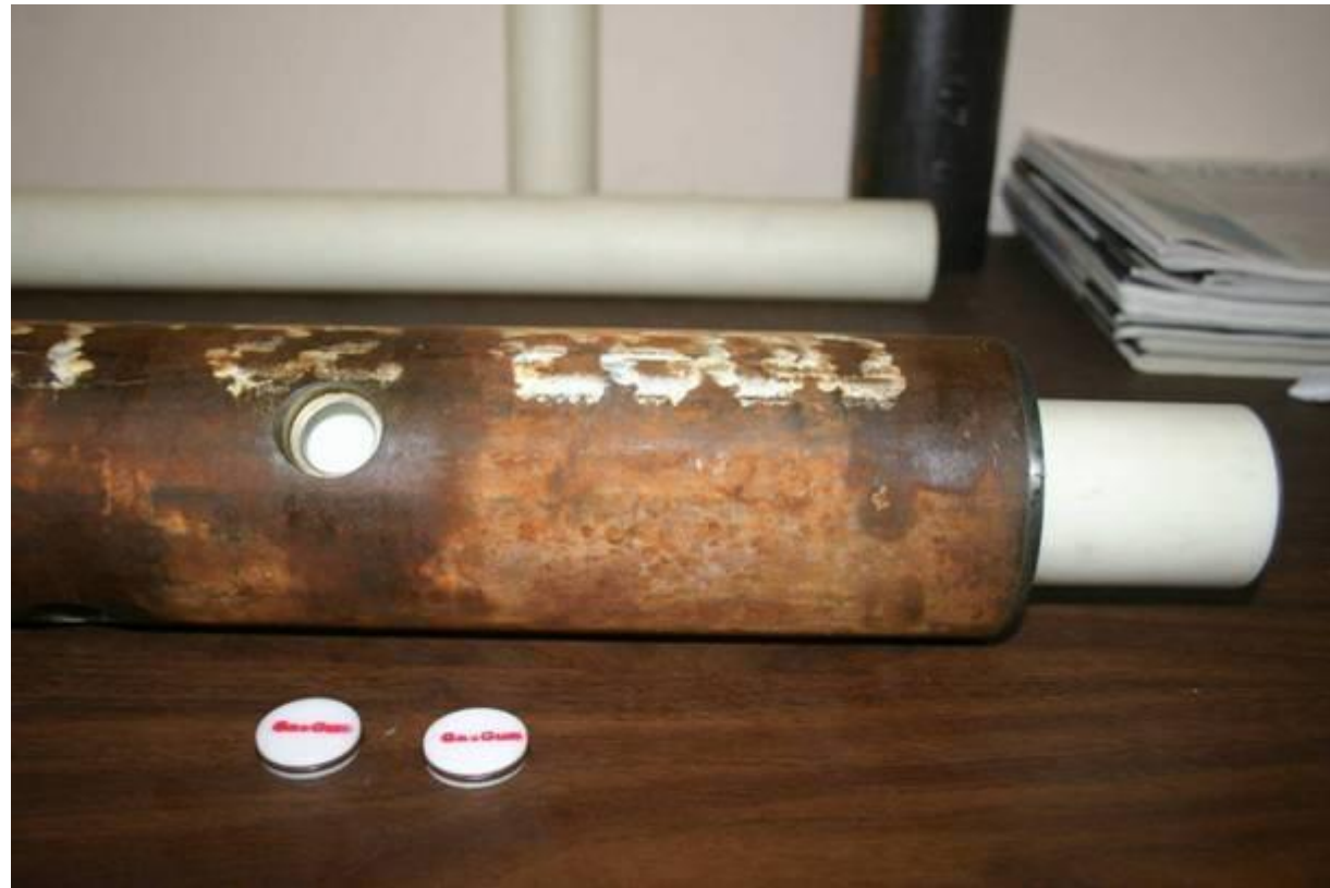
Hollow steel carrier tool-for enhanced pressure and temperature resistance
